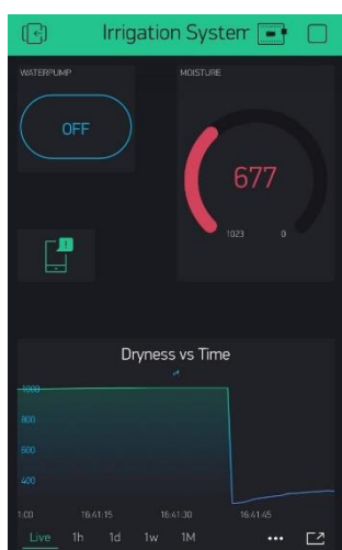
Fig. 21 – Blynk Interface during Wet Condition
