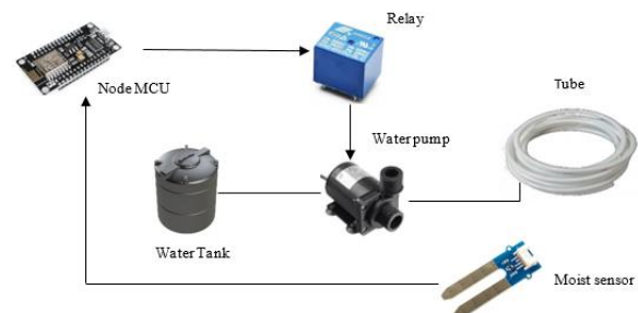
Fig. 7 – Block Diagram of the System Operation [10]
