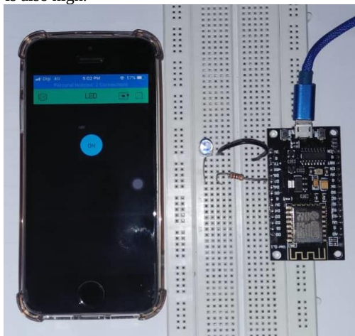
Fig. 8 – Simple Node MCU Connection
