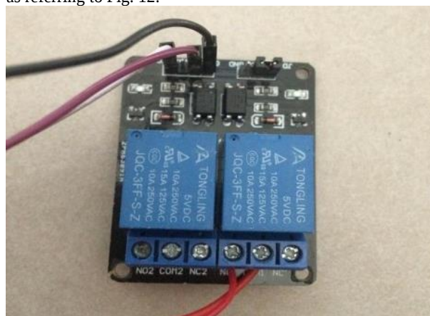
Fig. 11 – Relay with no signal received
