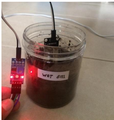
Fig. 15 – Moisture Sensor Module on Wet Soil
