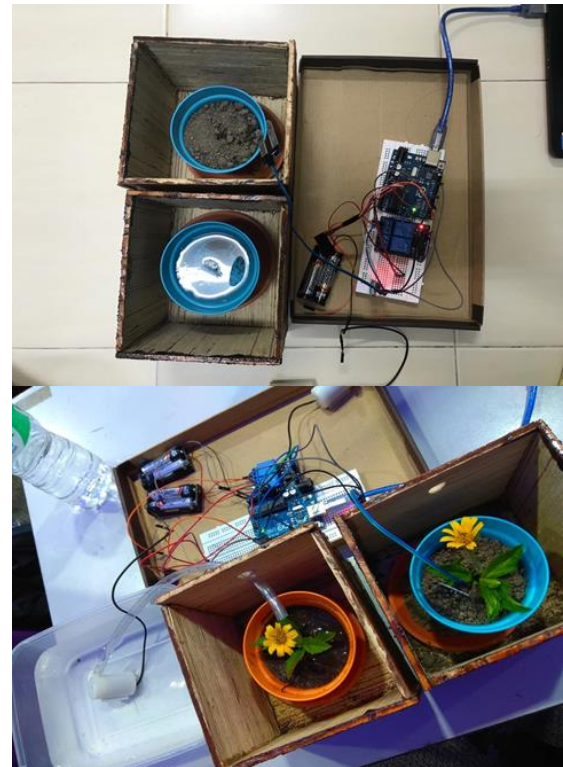
Fig. 9 – The prototype of IoT Plant Watering and Fertilizing System
