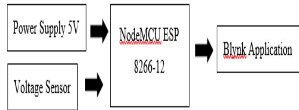
Fig. 13 – Block diagram for NodeMCU ESP 8266-12
