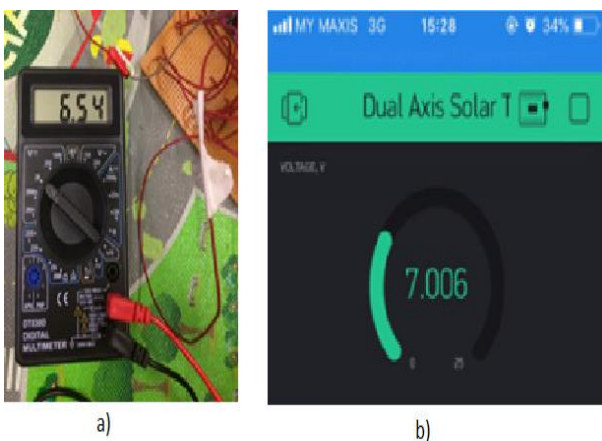
Fig. 19 – Dim weather condition reading, a) Direct voltage output from panel, b) Voltage output from system sensor
