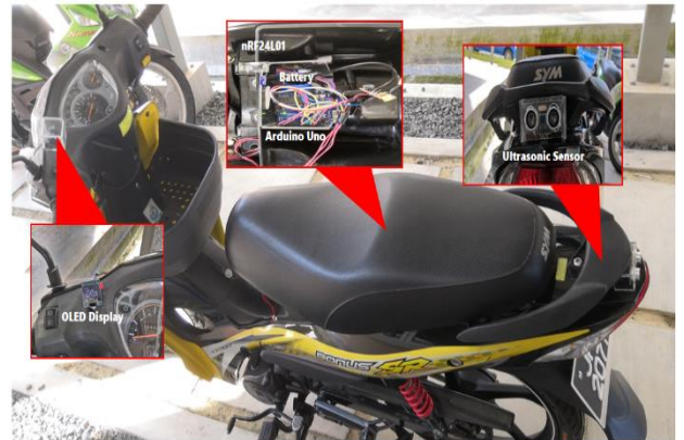
Figure 8: Implementation of transmitter unit at motorcycle
