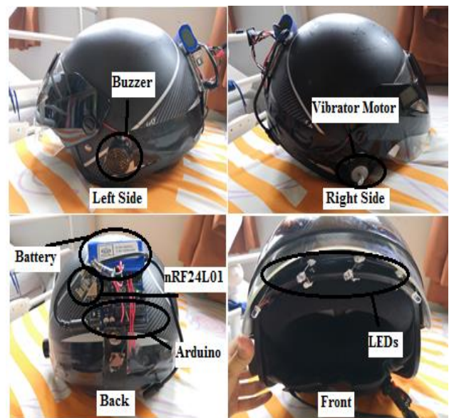
Figure 9: The smart helmet embedded with circuit receiver unit
